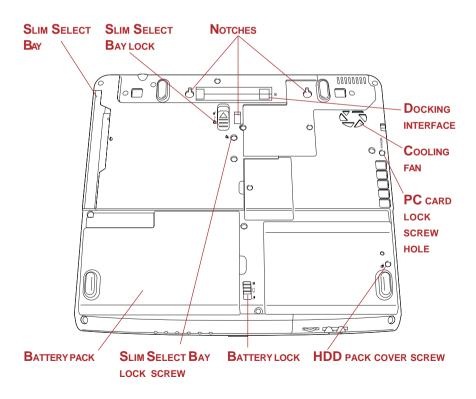
Figure 2-5 The underside of the computer
